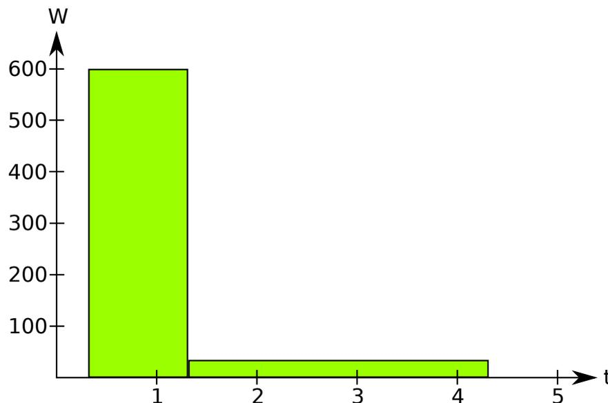
The energy of the first crank revolution is  $600 \text{ W} * 1 \text{ s}$ , or 600 J. The energy of the second revolution is  $66.7 \text{ W} * 3 \text{ s}$ , or 200 J. The objective for resampling is to have the resampled signal maintain the same energy content.
