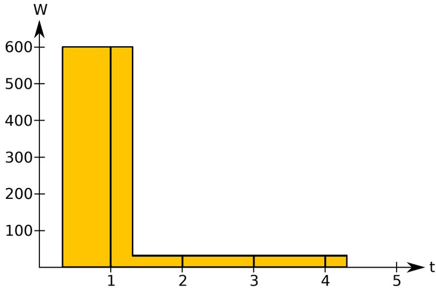
Now the energy in the first bin is 400 J, the second bin is 200 J + 44.4 J, the energy in the third and fourth bins is 66.7 J each, and the energy in the last bin is 22.2J. Because we are resampling to a one-second timebase, each energy is numerically equivalent to the average watts for that bin. So the wattage looks like this:
